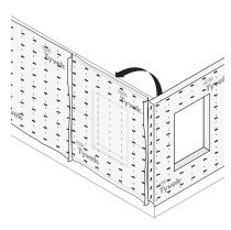
**STEP 6** After water-resistive barrier is installed refer to the DuPont™ Flashing Systems Installation Guidelines to prepare and flash windows and doors.
