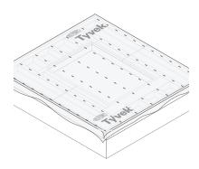
STEP 4 Fasten the side flaps and secure the bottom flap to the foundation. For maximum air leakage reduction (when installing as an air barrier), seal wrap at the bottom of the wall with DuPont™ Residential Sealant, DuPont™ Commercial Sealant, or recommended sealant, DuPont™ Tyvek® Tape, DuPont™ StraightFlash™ or DuPont™ Flashing Tape.
