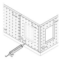
**STEP 2** When starting a wall section, fold the beginning side flap over the vertical side of the stud and secure. Trim off excess. Ensure that the bottom flap overhangs enough so that, when the wall is tilted upright, it overlaps the sill plate.
