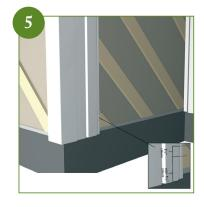
The base of the building should be measured so that the siding is no closer than 8" (203 mm) from the ground level. Please keep in mind that the siding must never touch the ground.
